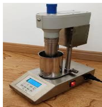
coquette type, coaxial cylinder rotational viscometer (model 286) Six Speed Rheometer –
